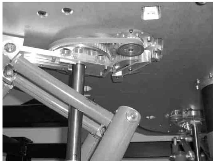
Figure 2.16. – Actuation system of each leg.
